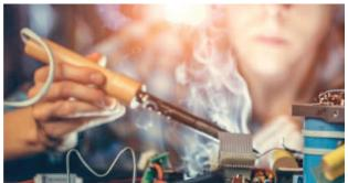
health risk (though makers should wash their hands if they've been soldering for long periods of time, or handling lead solder). Lead-free solder requires higher temperatures, can give off more toxic fumes, and is generally harder to work with, and for these reasons we don't recommend it.
